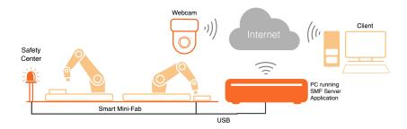
Fig. 4. Overview of the data flow needed for remote access. Additional modules are highlighted in dark orange.
